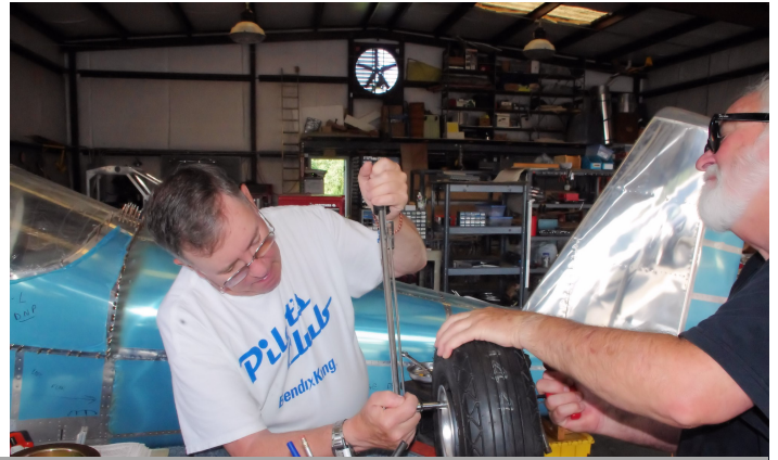
The wheel halves get torqued before being placed on the axle.
