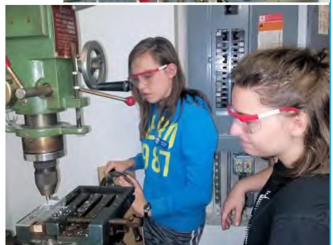
ShyAnne and Maddie milling the clearance slots for the control cables
