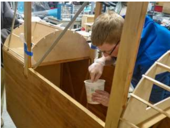
Applying Epoxy Varnish on the inside of the Fuselage
