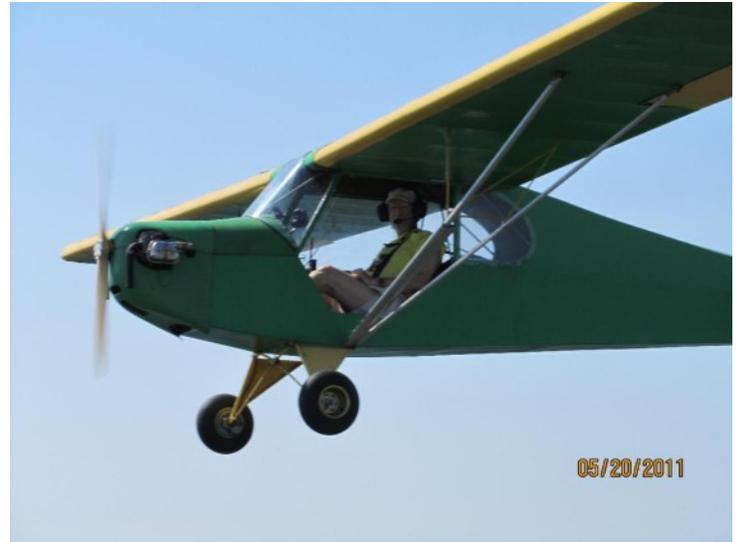
Hummel 37 hp half VW motor, 165 hours total time aircraft and engine. Cruise at 60 mph burning 2 gallons of car gas per hour! Land at 30 mph.
