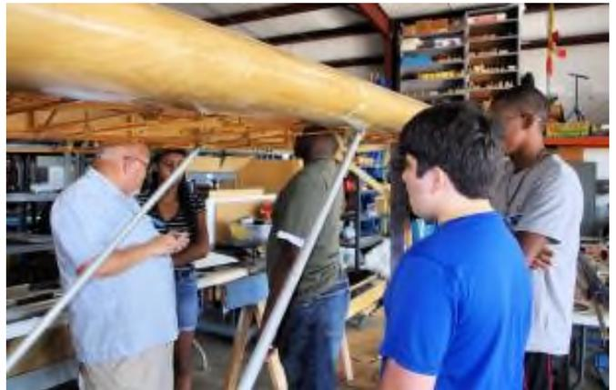
The struts are just about finished for the ultralite Piet. Next are the aileron control cables.
