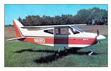
builder while utilizing the same German-made Hirth engine originally used in the BD-5. This high wing all-metal ship seats one person in an enclosed cockpit and stands on non-retractable tricycle gear .
