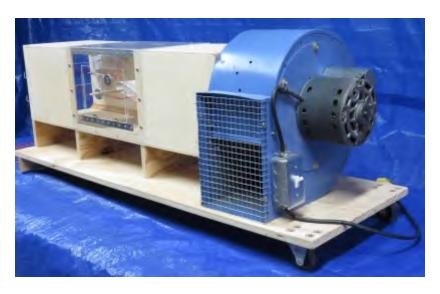
Also, with the idea of portability in mind he has rollers under the heavy blower end and a handle on the intake end so he can be rolled around much like a hand truck. Furthermore, because the blower motor end is flat and placed in the same plane as the end of the base, he can be stood up with the blower down in a stable storage position.
