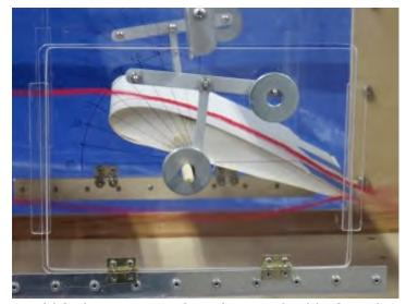
thereby indicating the amount of drag. To get the total lift the wing needs to be weighed before the test and this value is added to the weight of the washers used.
