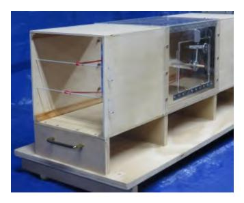
The airflow through the tunnel becomes visible by using red yarns suspended on rods across the intake of the tunnel. There are 9 sets of holes on 1 inch centers at the intake end which allows placing any combination of the available 6 rods and yarns (one or more rods with one or more yarns per rod). The student can choose whatever yarns (to include none) they wish while doing their test.
