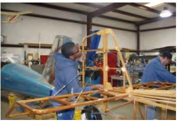
Adding the rudder for another control test
