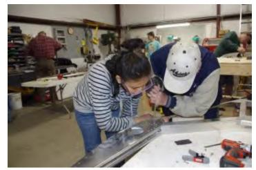
Most of the BD-6 goest together with machine screws
