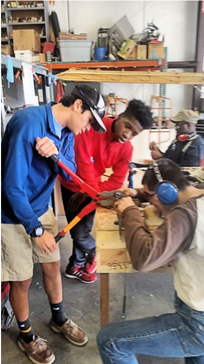
Alex ready to squeeze the Nicopress sleeve as Paul aligns the cable and Learch observes
