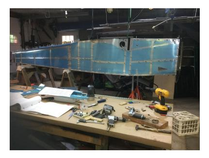
Here's a pic of my isolation therapy. The tail cone section is riveted and the mid and forward sections have been cleco'd and ready for final riveting.
