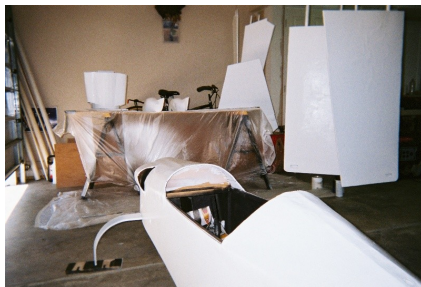
Custom built wheel pants of cardboard, plastic soap jug and paper mache
