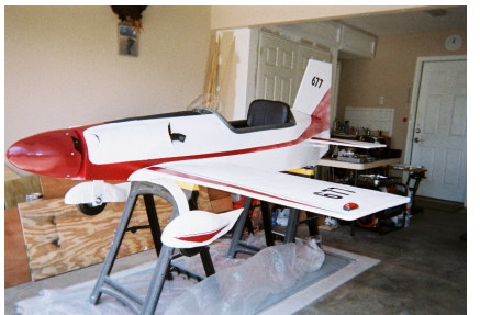
Custom built wheel pants of cardboard, plastic soap jug and paper mache
