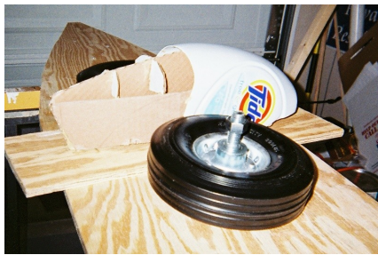
Custom built wheel pants of cardboard, plastic soap jug and paper mache
