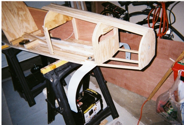
Fuselage, aluminum gear and wings coming together
