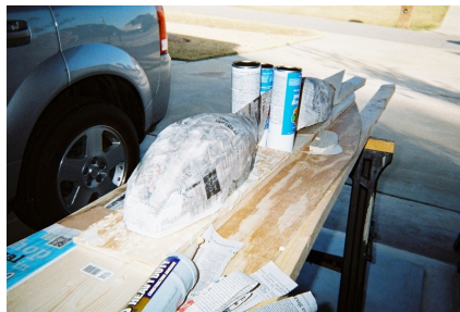
Custom built wheel pants of cardboard, plastic soap jug and paper mache
