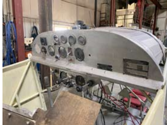
The Panel and fuel tank are in place.
