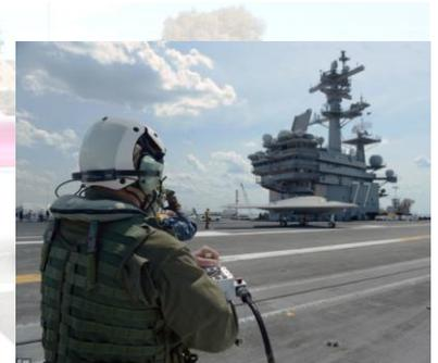
Fully autonomous: Mr Lorenz, Northrop Grumman's deck operator, drives an X-47B using his arm-mounted controller. It is fully autonomous in flight, relying on computer programs to tell it where it to go unless a mission operator needs to step in. The Pentagon has promised that it needs human intervention in order to open fire.
