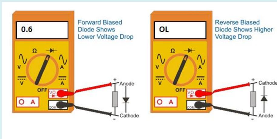
Diode defects can be either open or short. Open diode means diode behaves as an open switch in both reverse and forward-biased conditions. So,
