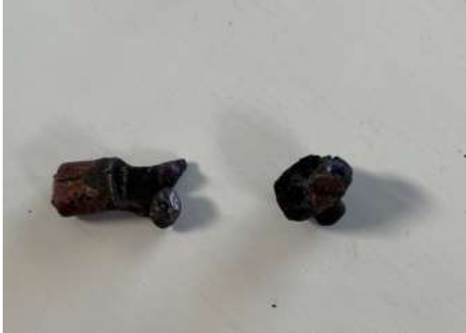
The melted away Wire Terminal, Stud and Nut
