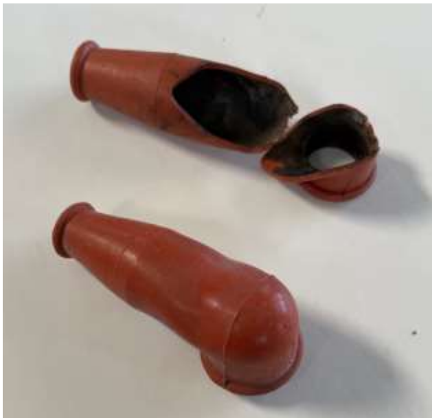
Looking inside the burned metal inside the boot
