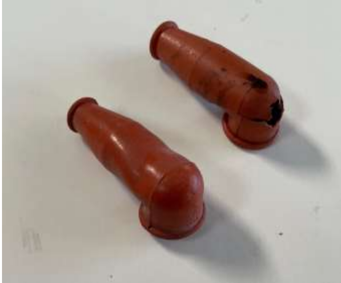
Upper Boot with Burn Through compared to the lower New Boot
