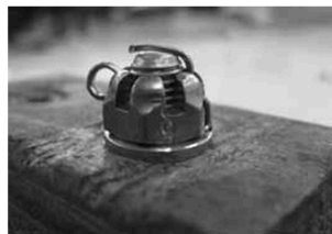
Fig. 2 (Correct Cotter Pin Installation)
