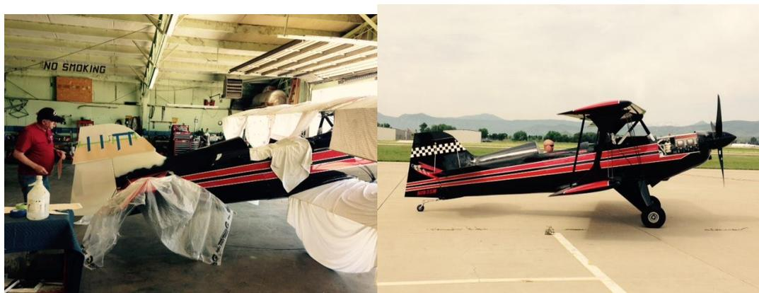
Brian had flown many Skybolts. N193SM is a Skybolt on steroids! Clipped wings, open front passenger seat, closed aft pilot seat with a whopping aerobatic, fuel injected, opposed cylinder, 540 cubic inch, 310 horsepower engine, designated as an AIO540. This monster engine swings a three bladed composite MT constant speed propeller and consumes 14 gallons of fuel per hour at best cruise. All of this with only a 25-gallon fuel tank.
