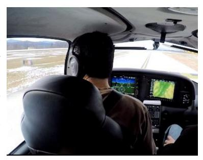
Finally, check your heading when you line up on centerline. If it doesn't match the runway number, either your directional indicator is not set, or you've taken the wrong runway. That's an easier mistake than you'd think where two runways cross at a common starting point.
