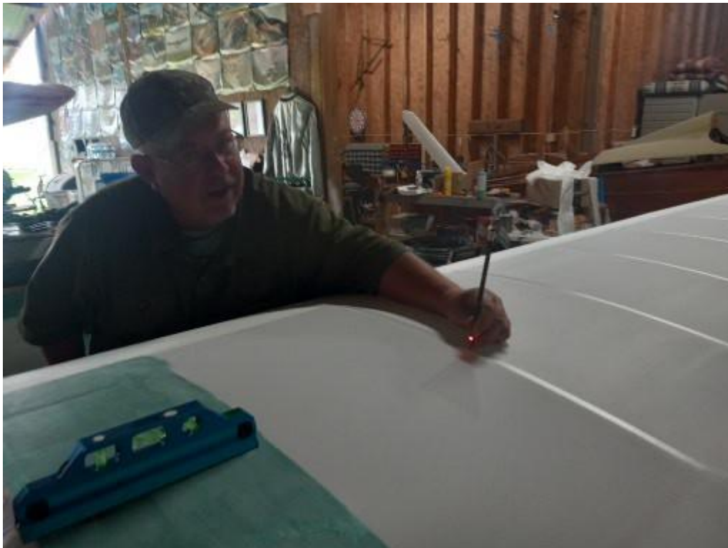
Al Bane lays out rib stitch spacing and alignment on the Fly Baby wing using a laser and pencil.
