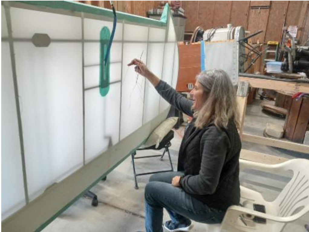
Casey Gabelli stopped by to assist with the rib stitching. Casey did a great job and learned a new skill. Kent Schmidt and Mike Lotz also assisted with the stitching. Much appreciated!
