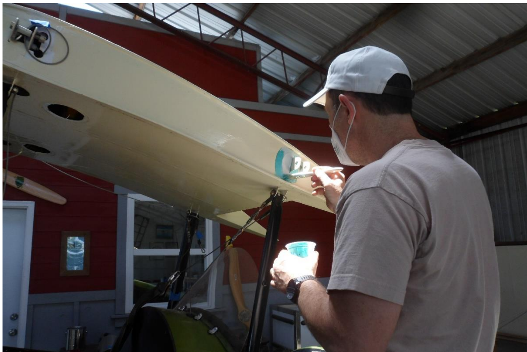
Bob Miller glues a fabric patch on the Scrounge Dawg Pietenpol wing center section.
