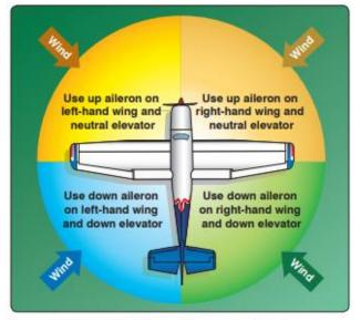
Figure 2-14. Control positions of the nosewheel airplane.
