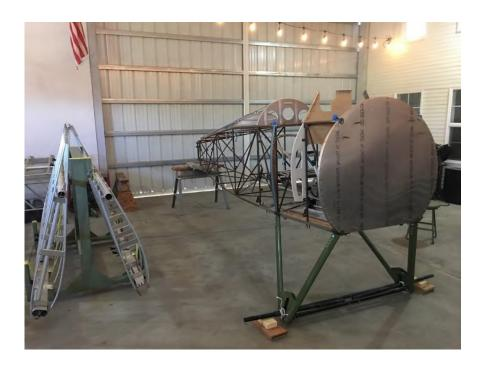
"Wings and tail off so I can build up the fuselage sides. Sides and top are aluminum panels from seat forward."
