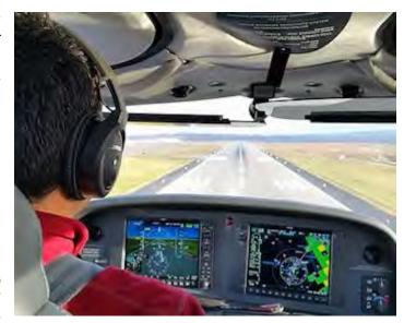
stable airspeed, I would go around early. If you can maintain airspeed, I would continue the approach and get into the wing-down technique early to confirm you can hold the centerline. Of course, if you can't, you need to go around.
