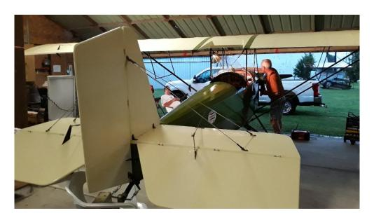
Tail sections repairs on the Scrounge Dawg Pietenpol were finally completed and reassembled.
