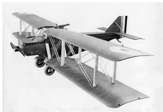
BOEING GA-2 GROUND ATTACK AIRCRAFT OF 1921 PLACED GUNS BETWEEN THE LANDING GEAR, FIRING FORWARD AND DOWN. (WALTER J. BOYNE COLLECTION)
