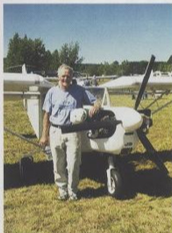
Red Rutkiewicz of Ravena, New York, built this Zenair CH 701 "from scratch, from plans," he says. He describes it as "really easy to build" and a nice airplane to fly. Completed in 1994, it's the third airplane he's built. Construction took two years. The cost was $4,600, not counting the 100-hp Continental engine, wheels, and instruments.
