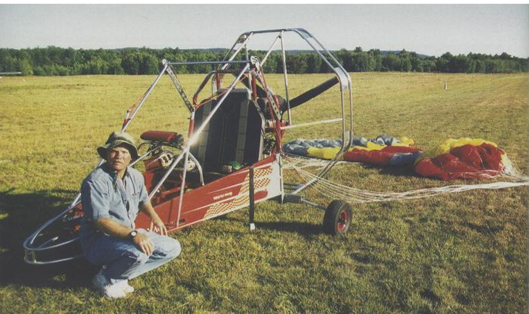
Viking Aircraft owner Charles Dozier of Panama City Beach, Florida, says he has more than 17,000 hours flying powered parachutes. He brought his company's side-by-side, dual-control powered parachute to the Mohawk Valley fly-in. He says they started out with a tandem unit in 1993, but that the side-by-side configuration, with its wide stance and low center of gravity, has greater stability and control in ground operations.
