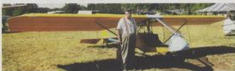
Mike Alexander, president of USUA Club 16, built this Rotax 447-powered Kolb FireStar and has been flying it for about five years. He's nearing completion of a 7/8-scale ultralight version of a World War I Nieuport fighter and expects to be flying it soon.
