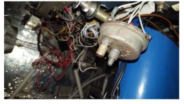
The original Stinson ignition/start switch was replaced with key type switch.
