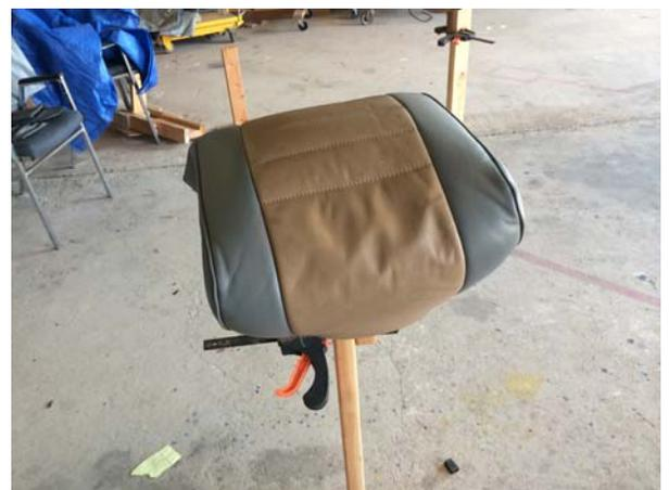
with the elastomeric paint and the seats, photos show the darker grey applied but had some lifting issues when the masking was done for the lighter gray (where the tan still is), paint and seat covers were shipped back to the manufacturer's lab to resolve the issue. Still has a few things to do yet; repair of the corrosion in the tailcone, landing
