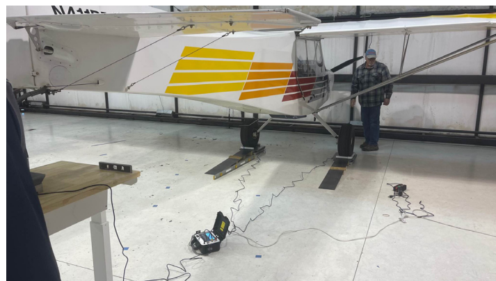
Patrick taking a final look at things and making sure the plane is ready to be weighed and the data will be accurate
