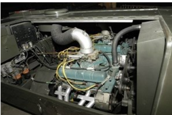
A view of the drive belt connecting the two engines
