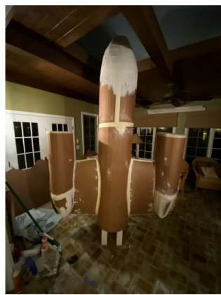
Built to compete in the Glen Ellyn Cardboard Regatta the entire aircraft had to be made from corrugated cardboard.
