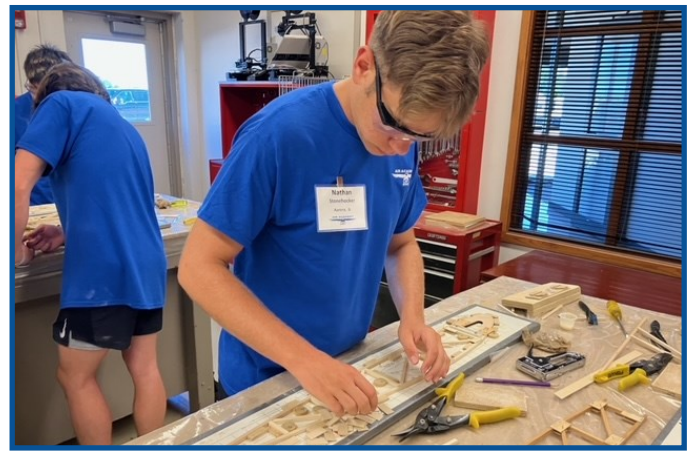
Working on a wing rib
