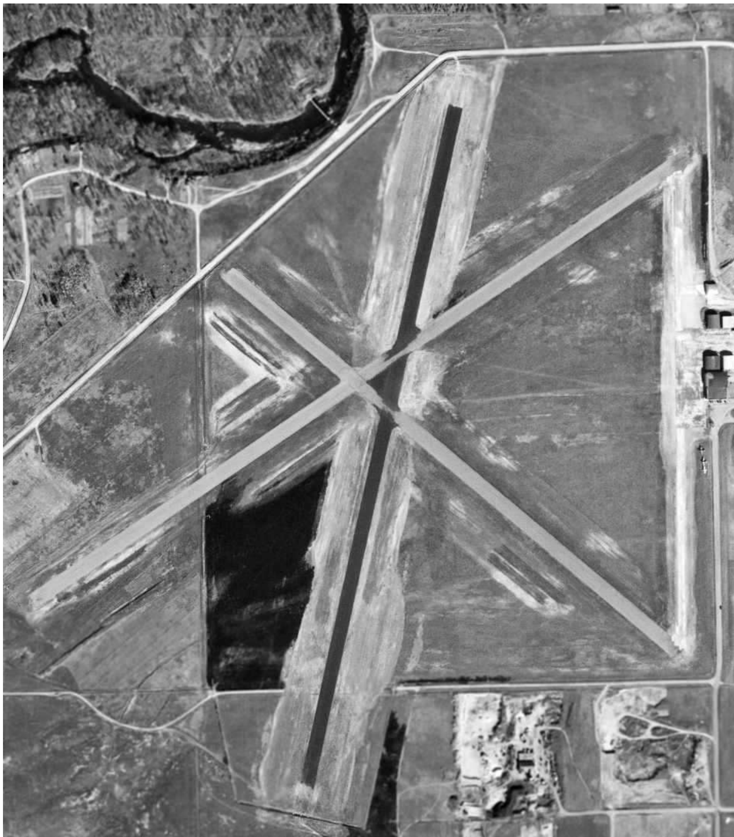
A 10/16/49 aerial photo (courtesy of Dallam Oliver-Lee) appeared to show 3 paved runways under construction at Whitney Memorial Airport.
