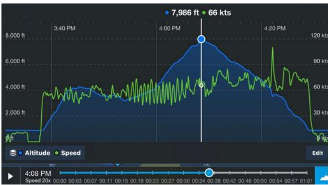
Fig 3: ForeFlight track log. Note the wiggles in the green ground speed line. That's from circling with about 15 kt of wind aloft. The speed spike at 4:22 is a dive to do a windmill start, without using the electric starter.
