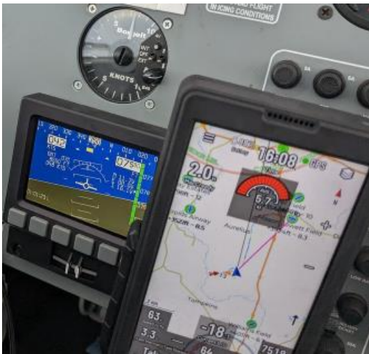
Fig. 4: 5.7 kt climb on the averager @ 7,500 feet. 7.5 on the vario, but near stall as I took the picture - would have been closer to 10 otherwise. (Hard to snap photos with climb turbulence, solo). Remember 1 kt = 100 fpm. Taking into account my sink rate of 400 fpm in a turn, air was rising at up to 1,400 fpm!
