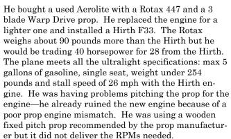
A 2 stroke engine needs to spin to its max rpm when the engine throttle is wide open. If it spins too high there is not enough load on the engine and the engine will eventually fail. If the engine spins too slow at wide open throttle—the engine is not producing all the horsepower it could produce and the exhaust gas tem-
