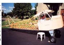
The airplane is an all wood, fabric covered, high wing, tandem seat two place Rotax powered homebuilt. It is a geodetically braced construction type, throughout, similar to some famous British designed airplanes of World War two. Bert Sissler, a well-known Minnesota amateur aircraft designer, used geodetic construction in his designs. He designed the Sissler's Whistler and the Cygnet.
