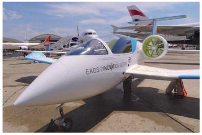
Its most unusual aspect is the ducted fan propulsion. Rather than use a <u>traditional propeller driven by an electric motor</u> like other <u>electric airplanes</u> we've seen (<u>and flown</u>), Esteyne uses a pair of motors with ducted fans — essentially small propellers within a cowling.
