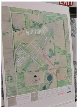
ing it to 3,600 feet. This would require moving the road at Gate A North and relocation the County Road South of the field around the end of the runway. The old 32 / 14 would be the taxiway for the new runway. Mac already owns land across the road from the approach end of 32.
