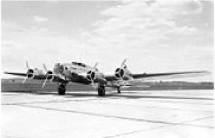
The Army continued to buy small quantities of upgraded B-17s (the A, B, D and D models) before the War. Thanks to the British, Boeing learned about the deficiencies of their design. Boeing developed the E model, which had the distinctive tail with its tail gun position. Actually, the tail was stolen from Boeings Model 307, and the tail was also used on the B-29.
