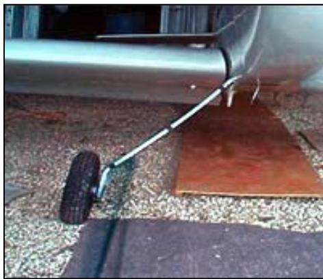
Damaged gear strut
