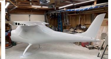
The Merlin is from a Czech company with beautiful and precise predrilling for rivets – he found only 2 holes out of 3500 that needed redrilling. The airframe kit runs \$18k, and the firewall forward kit is \$8k for the 60 hp HKS which is expected to give ~2.5gph eco cruise at 100mph, with a 120mph max cruise, running from a 6 gallon tank in each wing.
