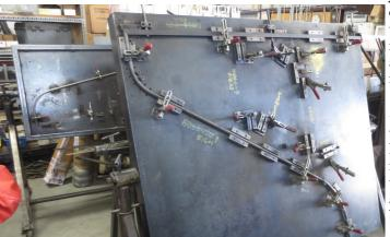
jigs to assure manufacturing efficiency and components of consistent dimensions and shape. Here is a tipoff to identify the current S7 John & Debra make from the earlier S7s. The rudder has been given a sharp rectangular corner at the top as opposed to the rounded off shape of the previous models – if you see a squared off rudder, it's the Super Sport.
