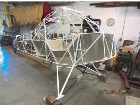
The fuselage of an Aviat float plane showed up on a flat-bed to have it's lower longeron repaired where the float mount had sort of taken the weld and part of the tube with it when it separated.
