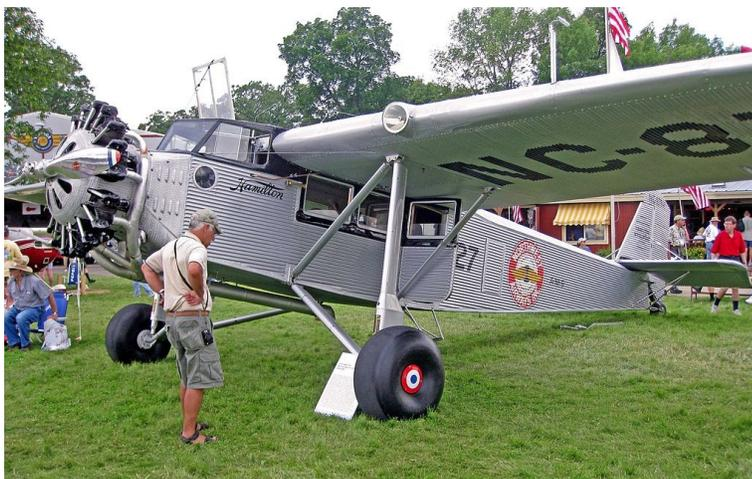
The corrugated skin, thick wings, and slab-sided fuselage of the Metalplane give the impression that the airplane might be a single-engine version of the Ford Tri-Motor, but it is not a Ford. These design features likely resulted from McDonnell's work for the Stout Metal Airplane Division of the Ford Motor Co., which designed and built the iconic Tri-Motor.
