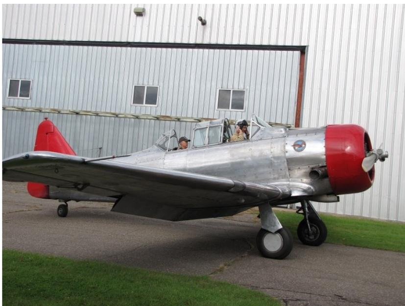
A 45-minute check out was part of the ride. Starting the 1,340 cubic inch 600 hp. Pratt & Whitney engine was just the best !The engine came to life with a clatter of noise, smoke, vibration, oil and exhaust fumes and finally a nice deep rumble as all nine cylinders began to fire. No doubt about it...there is a big engine up front!
