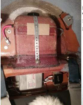
lowed me to hide the second transponder antenna there by getting creative with a virtual ground plane rather than a solid ground plane.
