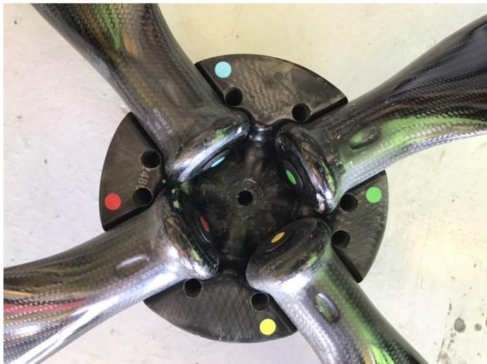
gear box as the engine sees very little of a load from the prop. The unique dihedral hub design angles the blades forward and uses centrifugal force to counter the effects of blade flex under load.
