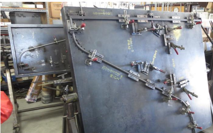
{photo 4} Kitfoxes use a single control surface attached to the trailing edge of each wing to serve as both flaps and ailerons; hence, the, the term “Flaperons” The factory does the shaping, assembly and bonding of the flaperons used on a Kitfox with the machine in the photo. The flaperons have a center aluminum tubular spar with foam ribs which are bonded between the spar and skin. The Flaperon brake serves the
