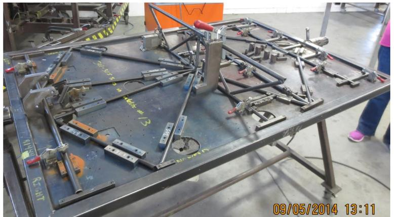
The factory has several operations being conducted in different buildings. The weldments are manufactured with various jigs to assure manufacturing efficiency and components of consistent dimensions and shape. Here is a tipoff to identify the current S7 John & Debra make from the earlier S7s. The rudder has been given a sharp rectangular corner at the top as opposed to the rounded off shape of the previous models – if you see a squared off rudder, it's the Super Sport.
