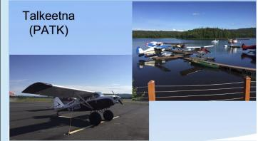
At Talkeetna Laura trained in a Piper Pacer with Tundra tires, practicing gravel strip landing, gravel bar landing, and avoiding gravel damage to the propeller and aircraft. She learned lighter colored gravel bar is dryer, and to overfly to check out, a second time to skim with wheels to feel firmness, to land the third time. During this time she was also studying for her commercial written exam. Denali provided great views and challenging airspace to fly in.
