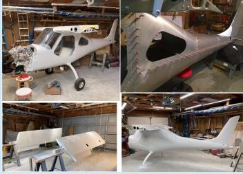
The Merlin is from a Czeck company with beautiful and precise predrilling for rivets – he found only 2 holes out of 3500 that needed redrilling. The airframe kit runs \$18k,
