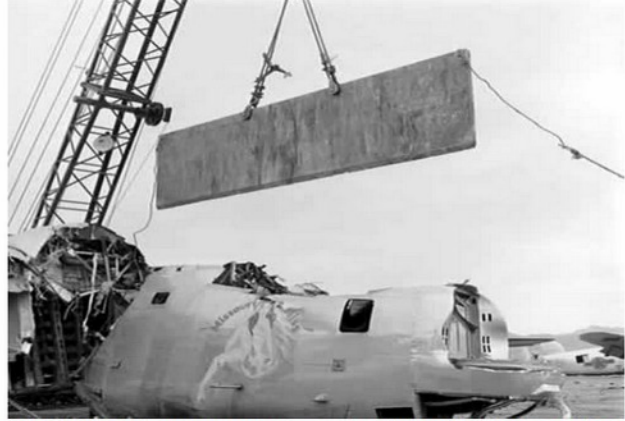
Consolidated B-24 Liberator "Missouri Miss" meets the guillotine at Kingman Army Air Field and Storage Depot 41
