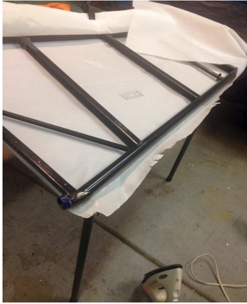
Making relief cuts for the ribs and bracing
