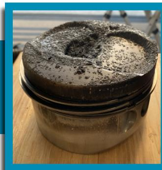
Severe detonation damage
