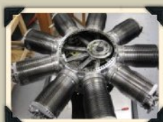
Detail of the rotary pistons mechanism in the Oberursel Engine.
